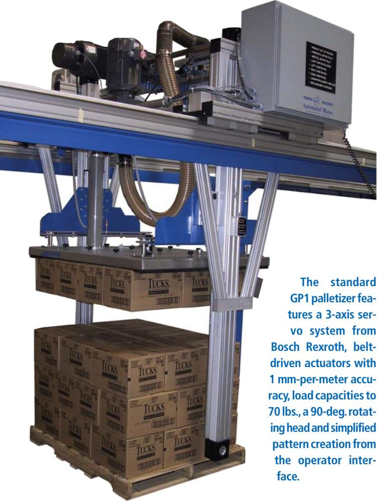
**The standard GP1 palletizer features a 3-axis servo system from Bosch Rexroth, belt-driven actuators with 1 mm-per-meter accuracy, load capacities to 70 lbs., a 90-deg. rotating head and simplified pattern creation from the operator interface.**
