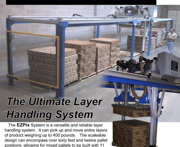
Choose to operate EZPix as a fully automatic gantry system, or in a semi-automatic mode with the operator pendant, as shown above. Either way, EZPix will increase your throughput while virtually eliminating ergonomic issues.
